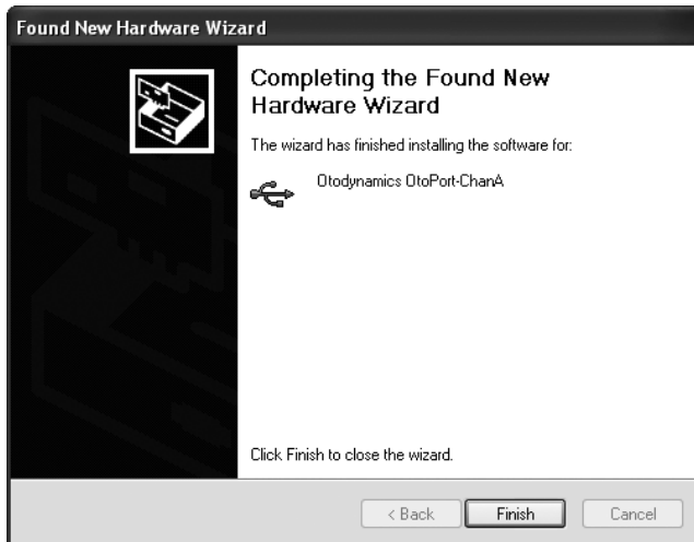
17.3.1.n Once complete click Finish . The driver installation for Otoport channel A is now complete and the same process is necessary for channel B.
